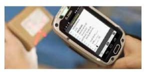
The new TC8000 mobile computer is the latest in its class (launched in 2016), and was designed from the ground up to increase worker productivity by 14%. Its innovative design minimizes the need to 'tilt and verify' enabling workers to more efficiently manage everyday processes such as; warehouse management, truck unload/load, pick/put away, replenishment, packing and shipping.
