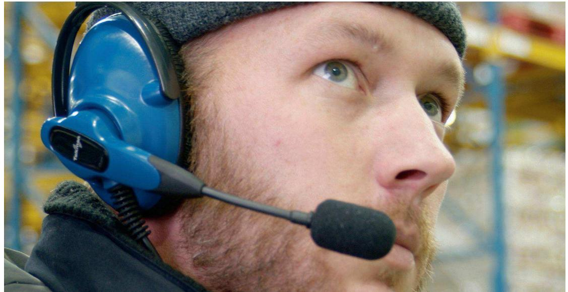
Speech recognition and RFID are alternatives to barcodes for accurate data entry, and have several advantages for cold environments. Speech recognition terminals are worn on a belt or shoulder holster, rather than carried, and can be worn under a coat. Terminals worn under coats aren't exposed to the temperatures cold enough to cause problems.
